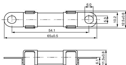
Mounting Torque: 3-5Nm
