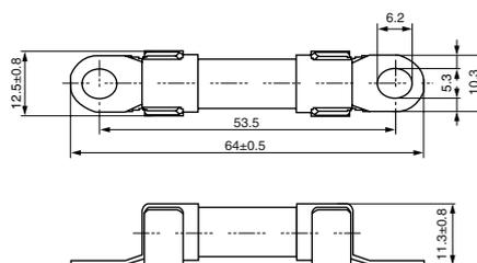
Mounting Torque: 3-5Nm
