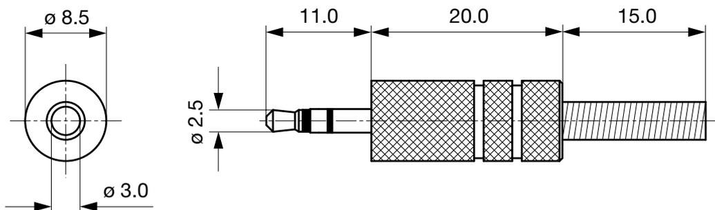
Cable diameter max. 3.0 mm
