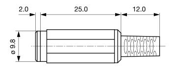
Cable diameter max. 4.0 mm
