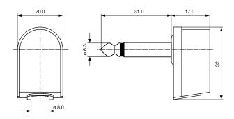
Cable diameter max. 8.0 mm
